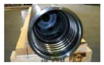
6. Pull the bit bearing from the hammer casing. Depending on the degree of rust or dryness in this area, a bearing puller may be needed for removal.
