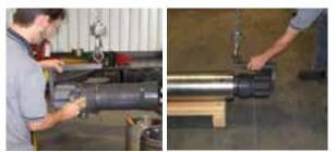
Lubrication and installation of the piston.
