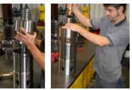
Installing the distributor in cylinder.
