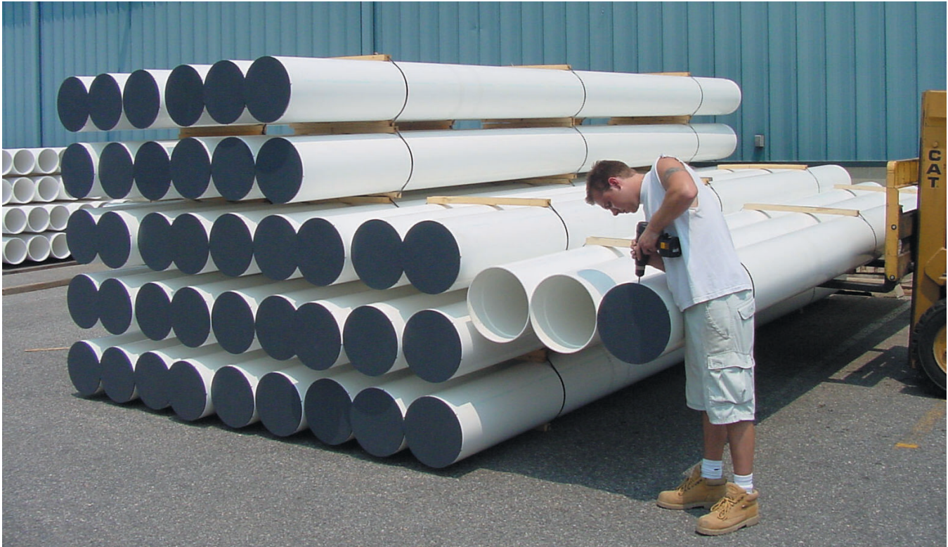
Elevator liner ready to be shipped from Forked River.
